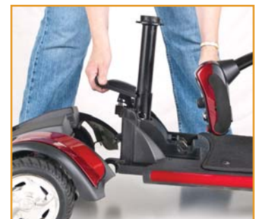
Step 3: Pull up on the drivetrain release lever to separate the front and rear frame sections!
