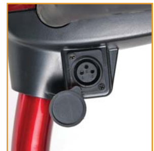
A battery charging port is conveniently located on the tiller under the control panel.
